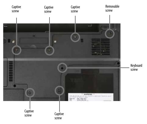
8 With a small Phillips screwdriver, remove the DVD drive screw, then put it in a safe place.
